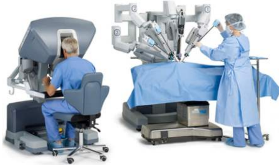
Figure 1.3: daVinci surgical robotic system. The surgeon sits at the console where his gestures are captured and converted to commands that control the slave-robot at the patient site. At the console the surgeon gets stereoscopic visual feedback. Typically these system have four robotic arms: one to hold the stereoscopic laparoscopic camera, two arms controlling surgical instruments, and one auxiliary arm. Image courtesy of Intuitive Surgical Inc.
