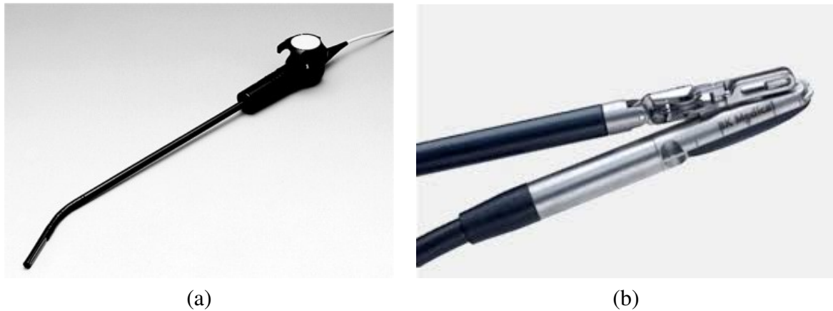
Figure 1.5: (a) laparoscopic ultrasound probe with an articulated tip. The linear transducer array provides a 2D US image while the manual controller at the handle enables articulation of the tip to reach otherwise difficult space, (b) drop-in (or pick-up) US probe with a curvilinear transducer array, designed specifically for robot-assisted surgical procedures. The probe has a grooved ridge that fits a laparoscopic/robotic grasper, enabling it to be picked up and manipulated. Image courtesy of BK Medical Systems Inc.
